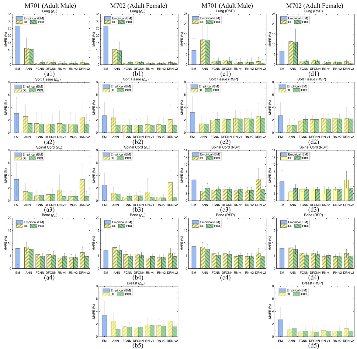
Figure 6. MAPE comparisons of mass densities between the reference and DECT parametric mapping models for a thoracic site from (a1)-(a4) CIRS M701 adult male and (b1)-(b5) CIRS M702 adult female phantoms. MAPE comparisons of RSP between the reference and DECT parametric mapping models for a thoracic site from (c1)-(c4) CIRS M701 adult male phantom with four tissue surrogates and (d1)-(d5) CIRS M702 adult female phantom with five tissue surrogates using a thorax TBDE scan.
