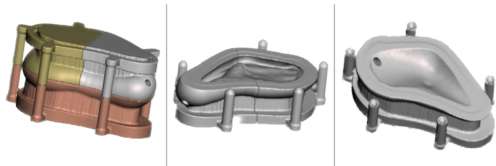
Figure 4. Virtual images of the designed mold using Meshmixer software (Version 3.5, Autodesk Inc., San Rafael, CA, USA).
