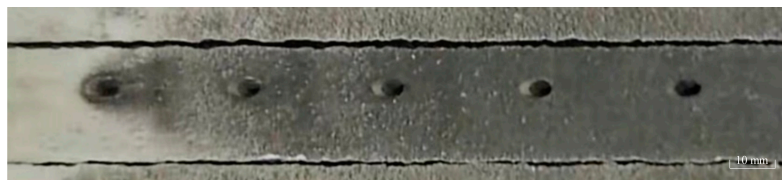
Figure 4. Sample after wire EDM.
