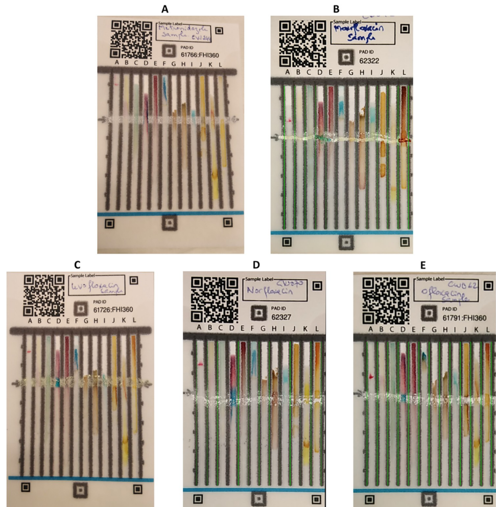
Fig 5. Cards of samples tested for specificity determination. A) testing of a metronidazole sample; B) testing of moxifloxacin sample; C) testing of levofloxacin sample; D) testing of norfloxacin sample; E) testing of ofloxacin sample. Lanes D and L were positive with blue and orange colors respectively for cards C (Levofloxacin sample), D (Norfloxacin samples), and E (Ofloxacin samples). The coloration of lane D for card B (Moxifloxacin) tends to green color.
