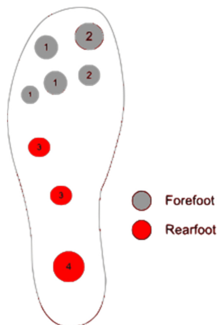
Figure 2. Location of the eight pressure sensors on the insole. Numbers indicating the different sensors and different colors are for the forefoot and rearfoot [19,29].
