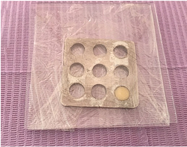
Fig. 1 Composite specimen preparation in a metallic mold between two glass slides and a nylon film. Each composite specimen was prepared separately in a metallic mold covered with a nylon film and held between two glass slides.
