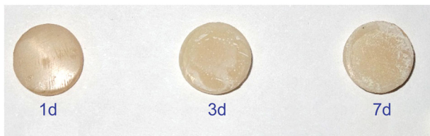
Fig. 6 The surface roughness of the samples after immersion in Dilsi Cola. The surface roughness of the samples increased after immersion in Dilsi Cola. The effect of the acidity of Dilsi Cola on the surface of the samples proportional with the time of immersion (1, 3, and 7 days).
