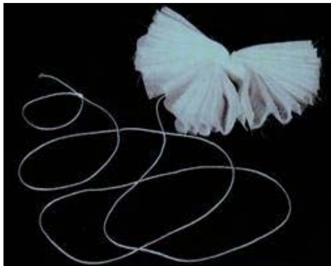
Figure 1. Moore Swab. A 4" by 4" gauze square, tied together with fishing line, which is suspended in wastewater for 24 hours.
