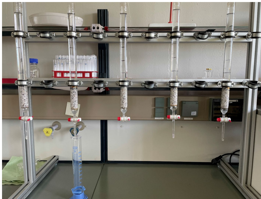
Figure 3. Column experimental set-up for \text{Fe}^0 leaching by ascorbic acid (2 mM). The photograph was made at the end of the experiments. The spout of the third column was broken during the experiments but this has no incidence on the performance of the system.
