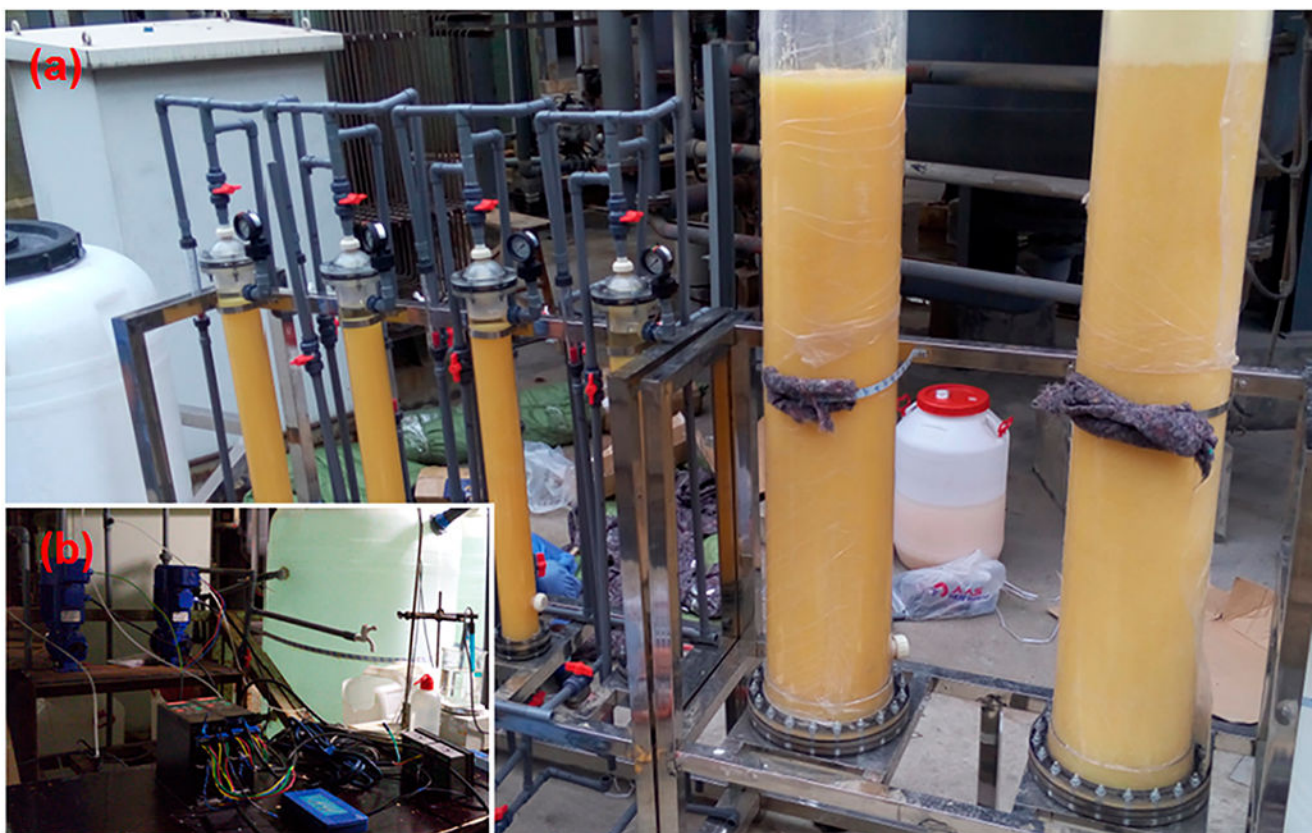
Figure 6. Purification system used in this work for the removal of iodine from salt water: (a) adsorption system and (b) control system. Reprinted with permission from ref 97. Copyright 2019 Elsevier.
