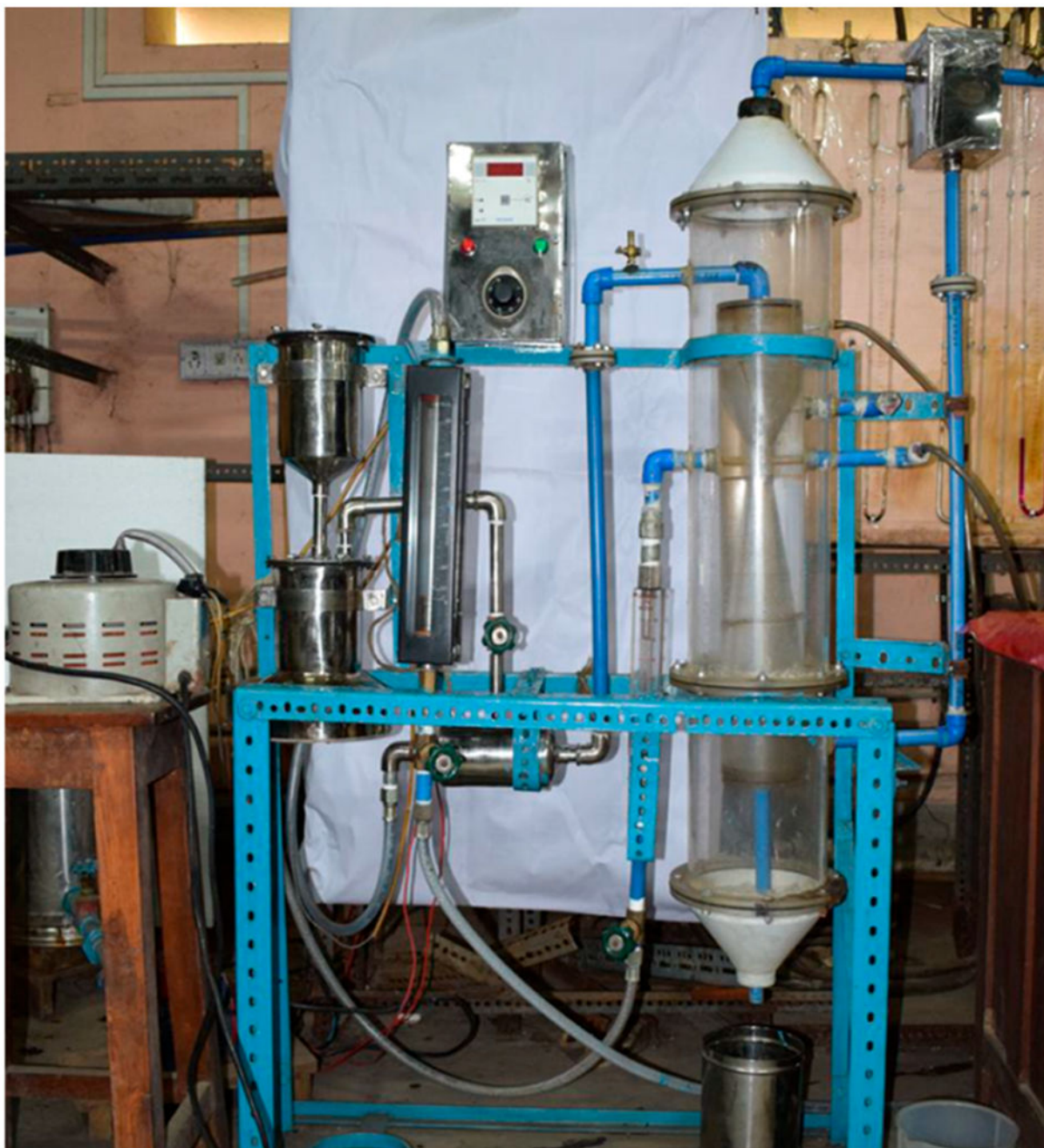
Figure 7. Picture of the experimental setup of a venturi scrubber using a filtered containment venting system. Reprinted with permission from ref 104. Copyright 2018 Elsevier.
