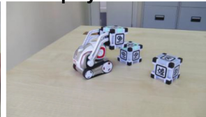
Figure 1. The social robot “Cozmo”. This robot can be used for embodied human-robot interactions in a wide variety of settings. Cozmo features face recognition of humans and pets, as well as the cubes, that are used in games and during free play of the robot. It uses facial, motion, and sound cues to communicate emotions based on an emotion engine that keeps track of internal- and external-triggered behaviour. The application associated with the robots allows for continues logging of events of the human-robot interaction. Photographs by Malte Heyen and Veronica Diveica.
