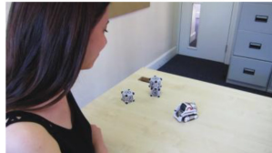
Figure 1. The social robot “Cozmo”. This robot can be used for embodied human-robot interactions in a wide variety of settings. Cozmo features face recognition of humans and pets, as well as the cubes, that are used in games and during free play of the robot. It uses facial, motion, and sound cues to communicate emotions based on an emotion engine that keeps track of internal- and external-triggered behaviour. The application associated with the robots allows for continues logging of events of the human-robot interaction. Photographs by Malte Heyen and Veronica Diveica.
