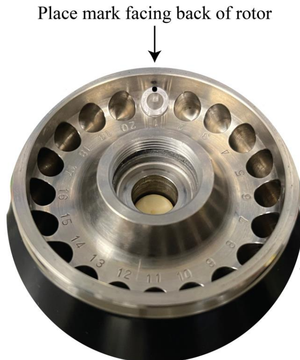
Figure 4. Example of how to orient the 7 mm × 20 mm tube in the S100-AT3 rotor
