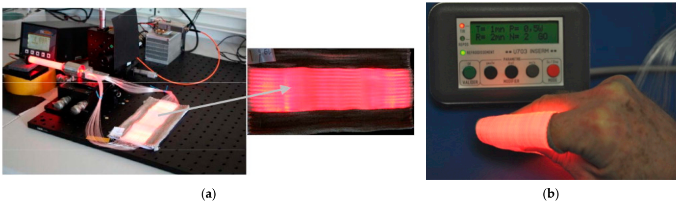
Figure 6. Textile light diffuser (a) connected to diode laser light source and (b) applied on a finger curved surface. Reprinted with permission from Ref. [132]. Copyright © 2012 Elsevier B.V.
