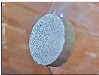
Figure 6. A representative natural titanium target utilized in the production of 47 Sc.
