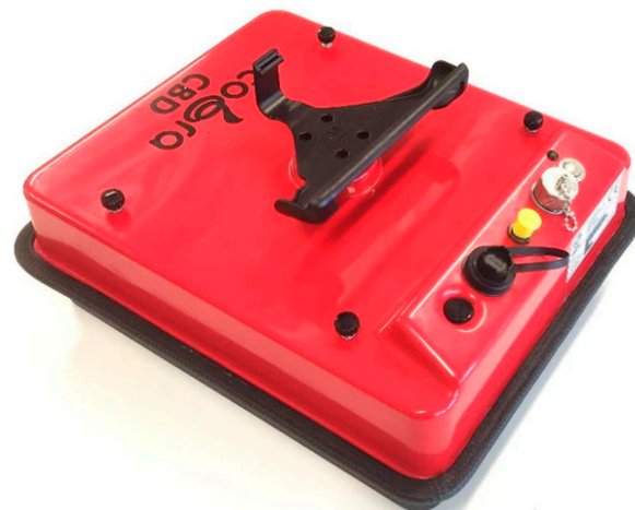
Figure 2. The drone CBD GPR that is in use with the DJI M600 pro [21].
