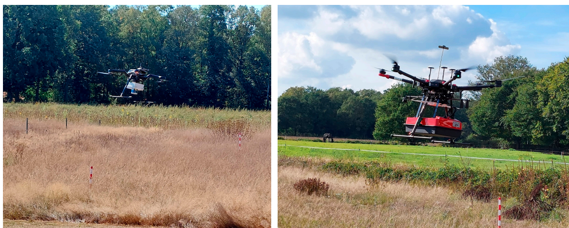
Figure 4. The left side of the figure depicts the Acecore Zoe used for obstacle avoidance. The right side of the figure depicts the DJI M600 combined with the GPR.
