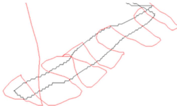
Figure 13. The red line depicted denotes the trajectory flown by the M600, which was integrated with the advanced RTK-GPS system. On the other hand, the black line denotes the route flown without the RTK-GPS system and highlights the lack of centimeter precision.
