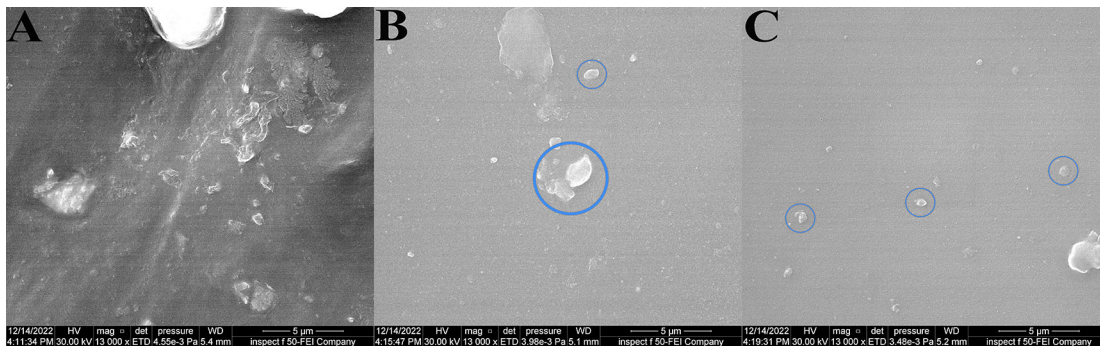
Figure 3. FE-SEM images at 13000 magnifications (5 μm) revealing evenly distribution of filler with a slight agglomerates as filler loading increases: A, control specimen; B, 0.5wt% specimens; C, 0.75wt% specimen. Circles show a number of large sized agglomerates of BaTiO 3 as filler loading increases.
