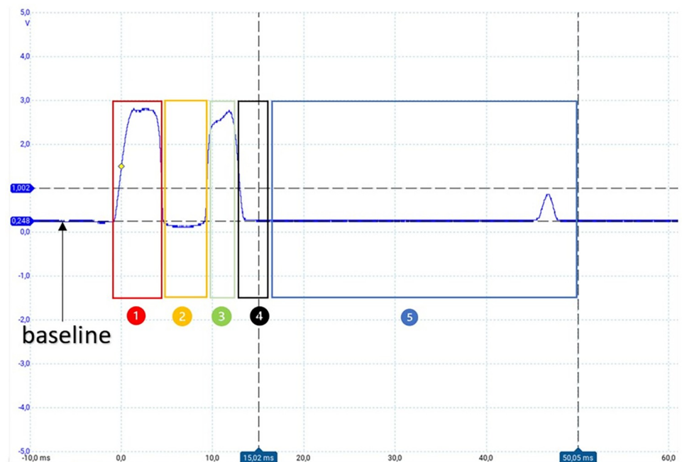
Fig 5. Pulse in detail of a normal drop. The numbers mark the different intervals.
