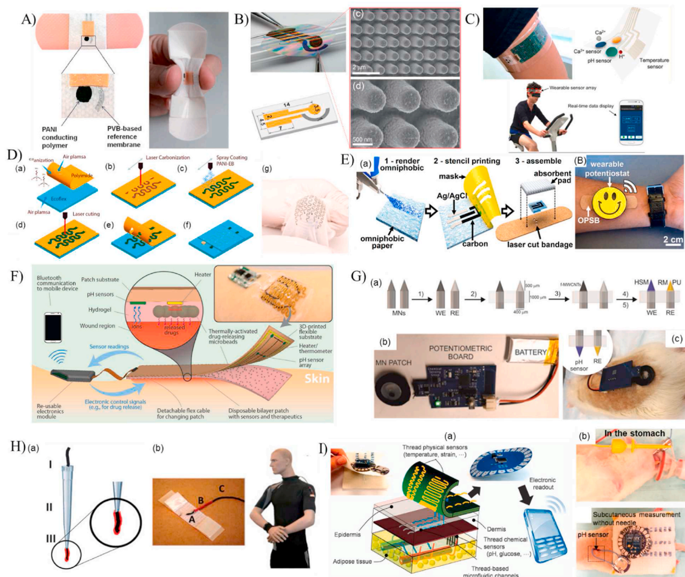
Fig. 3. Electrochemical based pH sensors. (A) A pH-sensitive bandage fabricated from PANI and Ag/AgCl electrodes [34]. (B) A PANI coated nanopillar array for enhancing the sensor's sensitivity [61]. (C) An integrated wearable pH sensor patterned on a flexible PET substrate and used for real-time monitoring of sweat pH during human activities [62]. (D) A high stretchable serpentine like pH sensor fabricated using laser carbonization of PANI [63]. (E) The fabrication process of the omniphobic paper-based smart bandages (OPSB) [64]. (F) An automated smart bandage for pH sensing and antibiotic drug release [65]. (G) In vivo transdermal pH sensing with microneedles electrodes [36]. (H) Details of the fabrication procedure of the cotton yarn-based band-aid [66]. (I) A toolkit of thread-based chemical and physical sensors, microfluidic channels, and interconnects for the realization of a thread-based diagnostic device [67]. (Reproduced from Refs. [34,36,61–67] with permissions from Wiley online library, Elsevier, ACS publications, pubs.rsc.org and Nature).
