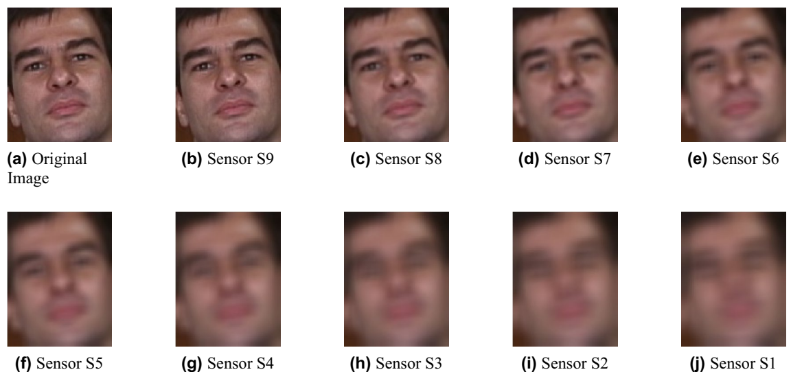
Figure 5. Example of synthetic images from the Georgia Tech Face database for each sensor at a distance of 5 meters.
