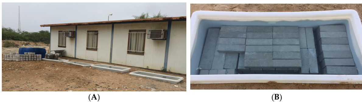
Figure 2. (A) Curing area of concrete samples (outside the laboratory), (B) freshwater curing tank.
