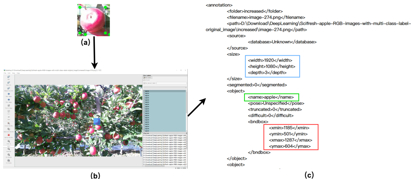
Figure 4. Labeling process: (a) a labeled apple; (b) annotation of an image; (c) annotation file: <size> denotes the length and width of the image and the number of channels; <object> denotes the category of the labeled object (“apple”); <bndbox> denotes the pixel coordinate position of the labeled object, which contains the upper-left and lower-right coordinates of the labeled apple.
