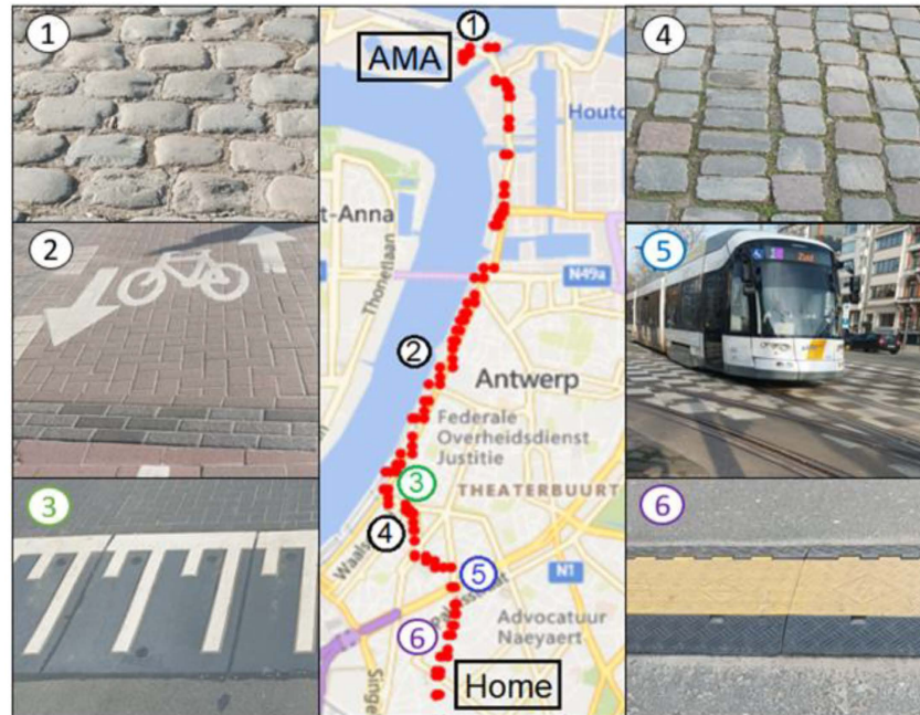
Figure 8. Journey of ca. 5.5 km from AMA to home using a bike at an average speed of 11 km/h together with the position of the events caused by irregularities in the road. The red dots stand for cyclist's position according to the GPS sensor GY-GPSV3-NEO-M8N. The numbered images at the left and right are associated to the numbered positions in the map and are related to the numbered events in Figure 7.
