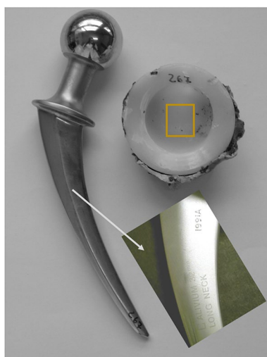
Fig. 1 Charnley–Muller Alivium monoblock hip implant with high-density polyethylene cup. Both femoral and acetabular parts are cemented. Inset shows the Alivium trademark
