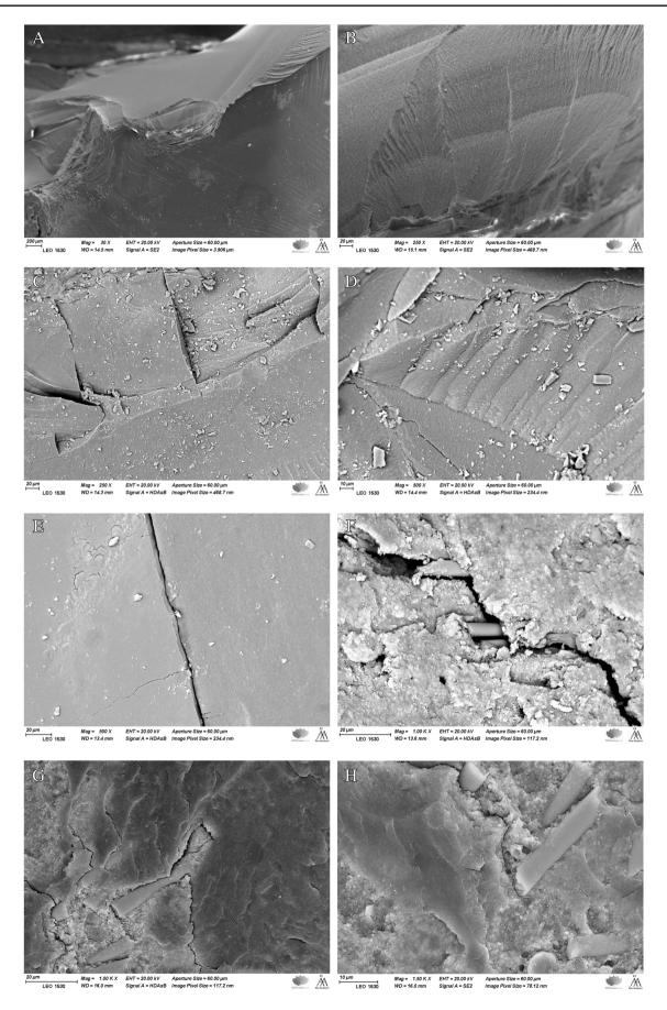
◄Fig. 5 SEM images of fracture surfaces of investigated bilayered structure restorations observed under different magnifications showing arrest lines with twist hackles (A–D, arrows) and a radial cracks (D & E) propagated through the restoration from the load application area to the SFC core. F, G, and H show short fibers' ability to redirect and hinder crack propagation (arrows)
