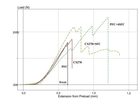
**Fig. 4** Load–deflection curve of representative specimens from direct and indirect restoration groups with and without SFC core
