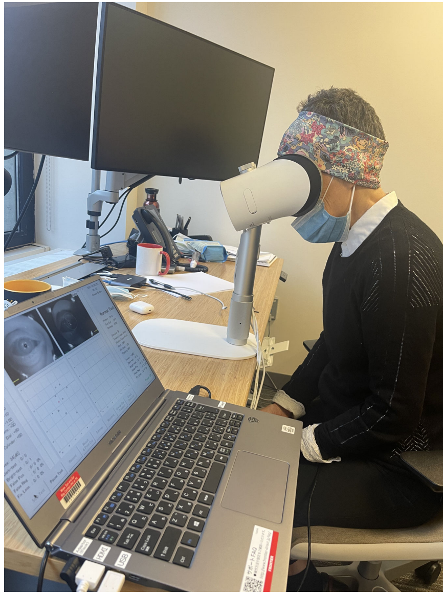
Figure 2. Smart Visual Function Analyzer (SVFA). (a) Components include: a headset (unit and portable stand), patient response button, test controller laptop, and set of spherical and cylinder lenses. (b) (c) Participant utilizing the SVFA. Photo release consent was obtained.
