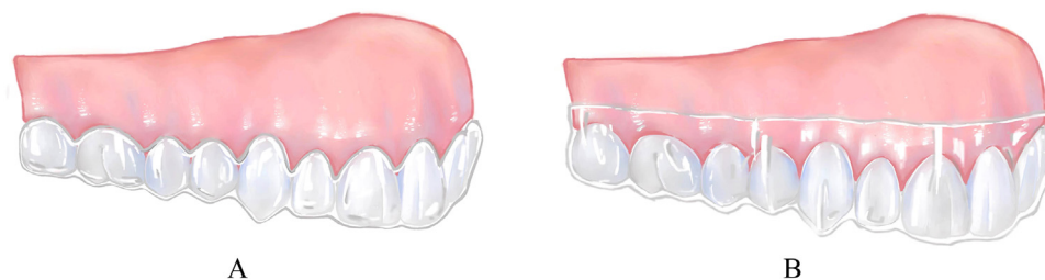
Fig. 1 – Two main gingival margin design features of clear aligners. A, The gingival margin of the aligner is designed as scalloped. B, The gingival margin of the aligner is designed as straight 2 mm up the gingival zenith.
