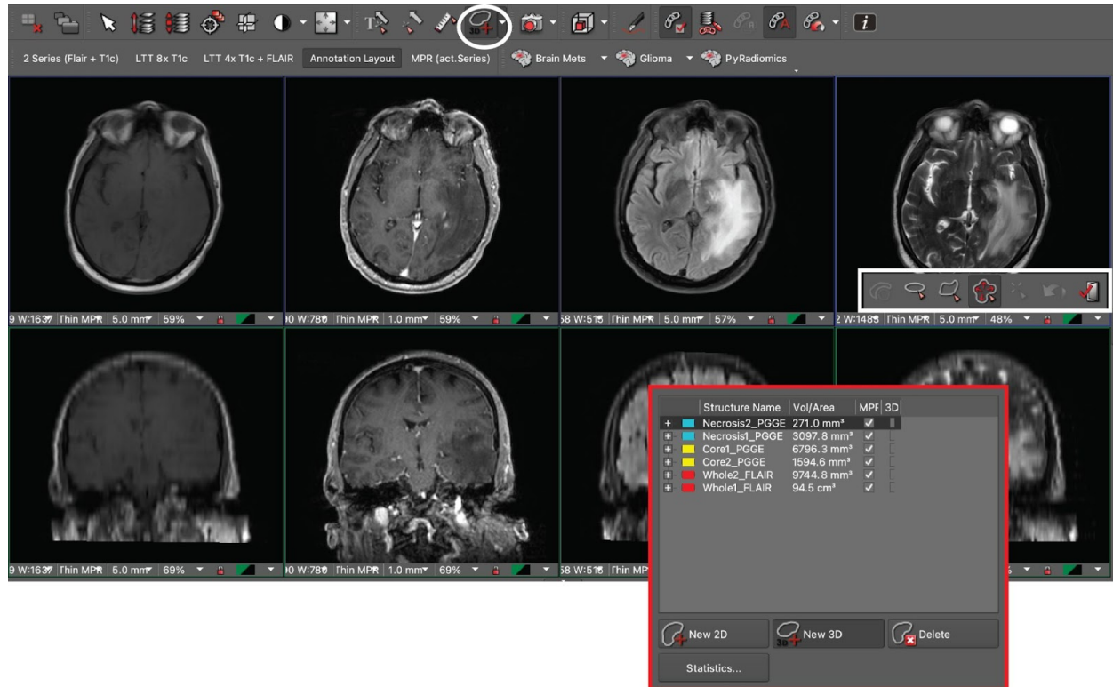
Fig 1. Research PACS annotation layout with T1, T1 post-contrast, FLAIR, and T2 sequences aligned. The PACS interface incorporates a 3D volumetric tool (white circle / rectangle) and displays labeled segmentations for two metastases in the display window (red rectangle).
