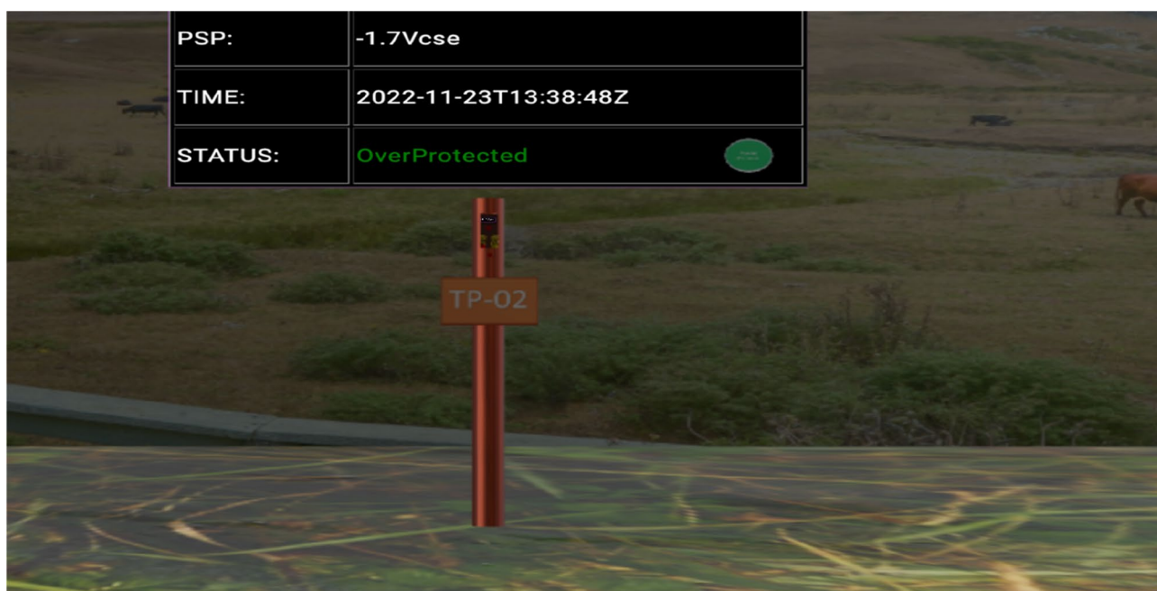
Figure 17. CPS remote monitoring display with over-protected status.
