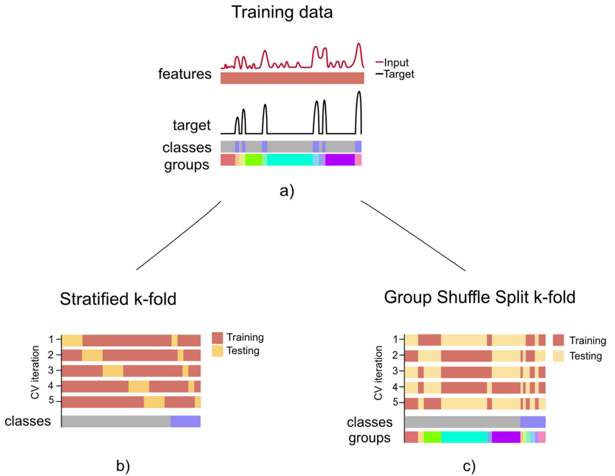
Fig. 4. Schematic representation of different k-fold cross-validation (CV) strategies. a) Training data, corresponding to an input vector of features (red) and an output target vector (black), e.g. movement trace, where two classes are involved and same sized groups are defined according to movement/no movement consecutive data chunks. b) In the standard stratified k-fold CV data is split into train and test sets, preserving class ratios in both sets. c) For invasive neurophysiological decoding we propose a group shuffled split k-fold CV strategy. While in the stratified k-fold CV class distributions are preserved along the CV iterations, features coming from the same group can be used for training and testing. The group k-fold CV ensures that group structure is preserved during training and testing set construction, but information about individual group blocks may not be preserved. For imbalanced class distributions data can either be rebalanced or cost function weights can be attributed class specific.
