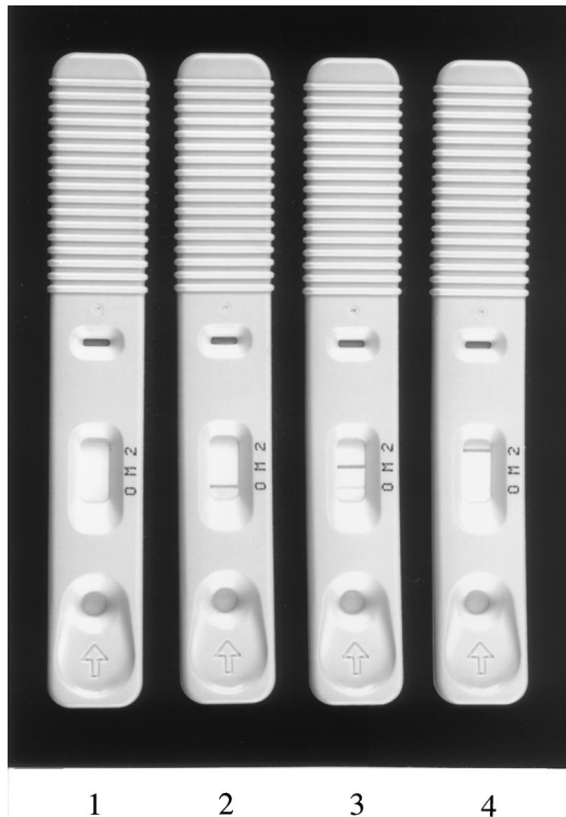
FIG. 2. Results of HIV rapid assay for control serum panel. Lane 1, negative control; lane 2, HIV-1 group O-positive control; lane 3, HIV-1 group M-positive control; lane 4, HIV-2-positive control.
