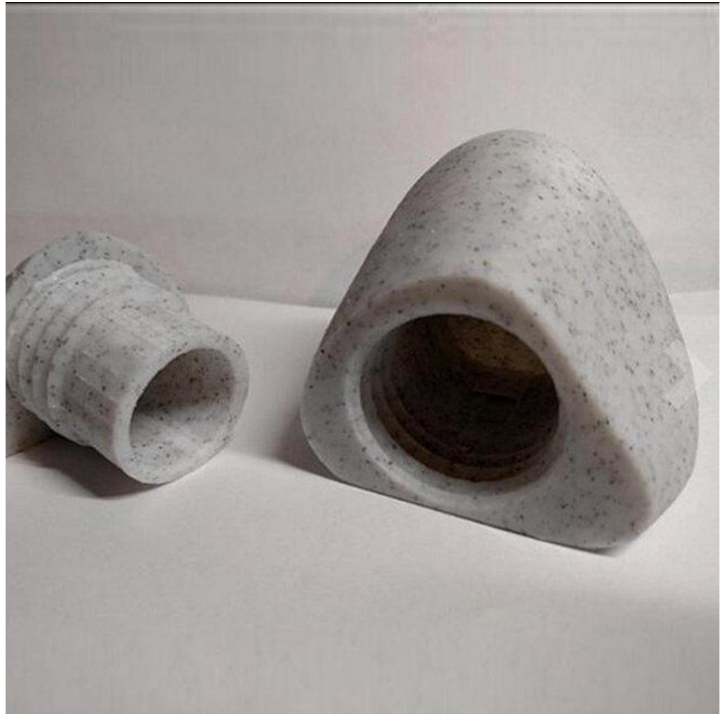
Figure 8. An image of 3D-printed items made out of ceramic-filled filament.
