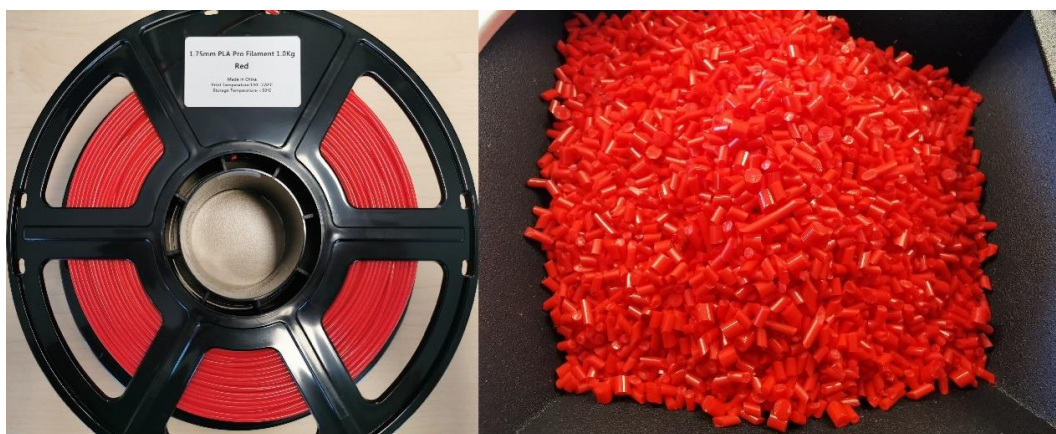
Figure 1. PLA raw material in the form of filament (left) and in the form of pellets (right).
