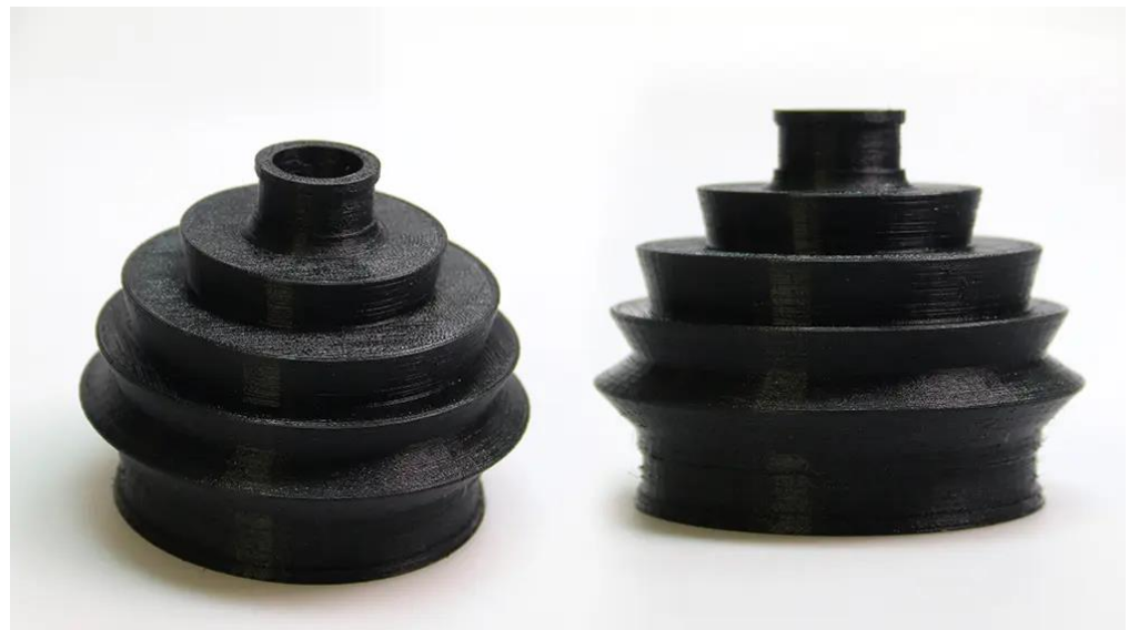
Figure 7. An image of 3D-printed items made out of flexible TPU-filled filament.
