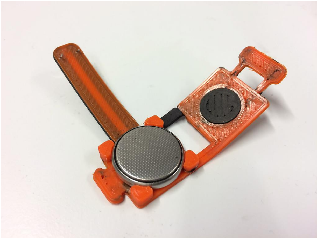
Figure 6. An image of 3D-printed items made out of conductive filament [100].
