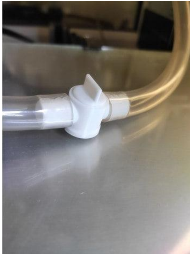
Figure 5. An image of 3D-printed items made out of glass-filled filament.
