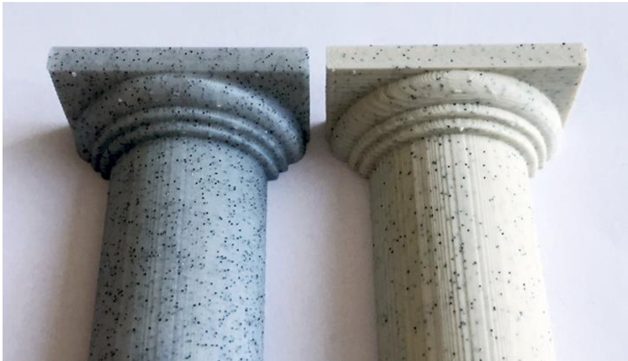
Figure 11. An image of 3D-printed items made out of stone-filled filament [135].
