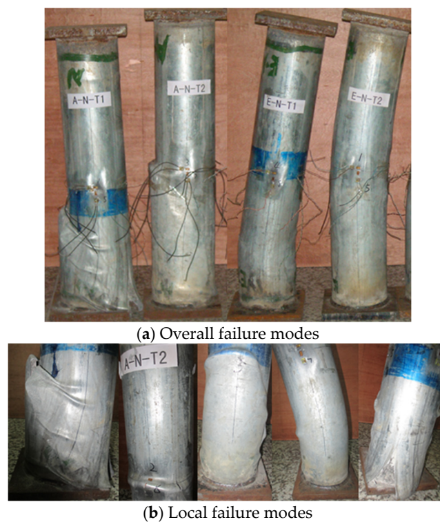
Figure 3. Failure modes of the columns.
