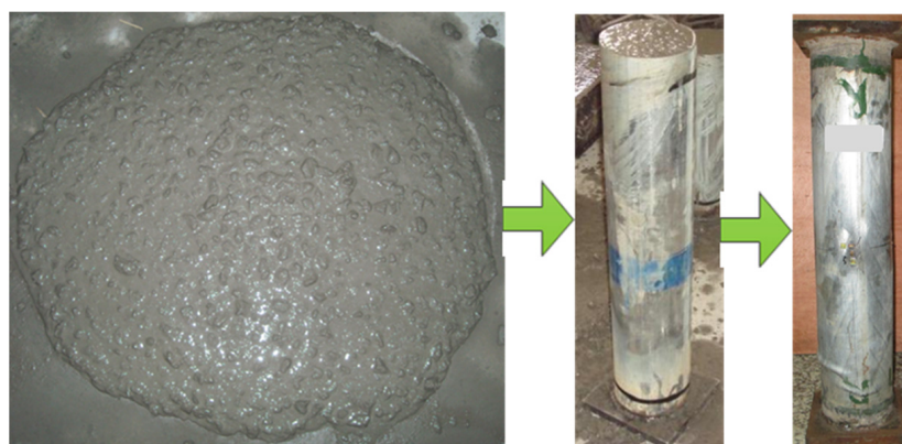
Figure 1. Preparation for the SCCTST columns.
