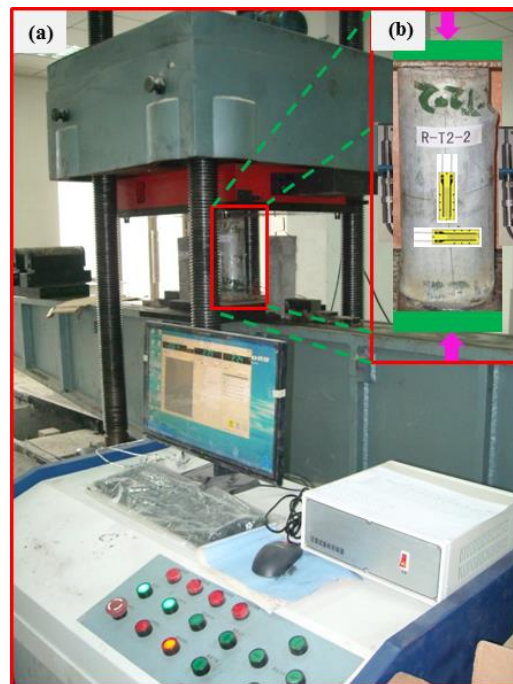
Figure 4. Photos of loading process of the columns. (a) The testing machine, (b) the columns subjected to compression.
