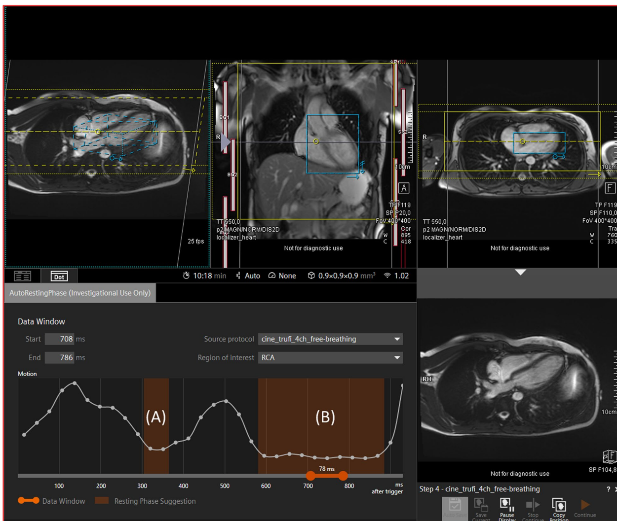
Fig. 1 Showing the process of scan planning and the degree of automation. Following acquisition and automated analysis of a free-breathing 4-chamber scan the DL-based software identifies both the end-systolic (A) and mid-diastolic rest (B) periods, which can be used to determine the acquisition window. The DL based software also determines the position of the coronal 3D imaging slab (in yellow) and iNAV box (in blue) to be used in the coronary MRA acquisition. The placement of the shim box and 3D imaging plane does on occasion require slight manual adjustment, especially in cases where the heart is larger than average
