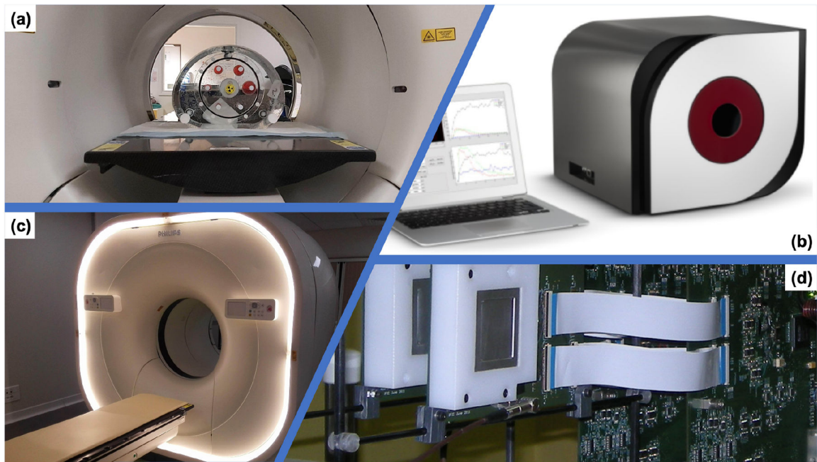
Figure 2. Examples of some simulated imaging systems (clinical, pre-clinical, prototype). (a) NEMA IEC Body Phantom Set ready to be imaged on a PET/CT. (b) The Bioemtech \gamma -eye preclinical device. (c) Philips Vereos Digital PET/CT; (d) MACACO Compton Camera prototype with 2 layers of \text{LaBr}_3 monolithic crystals coupled to SiPMs, developed by IFIC-Valencia.
