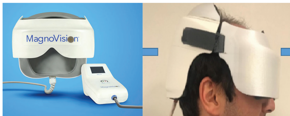
Figure 3. Retinal electromagnetic stimulator (Magnovision) device. Application of the helmet to stimulate the retina-optic nerve and visual pathways.
