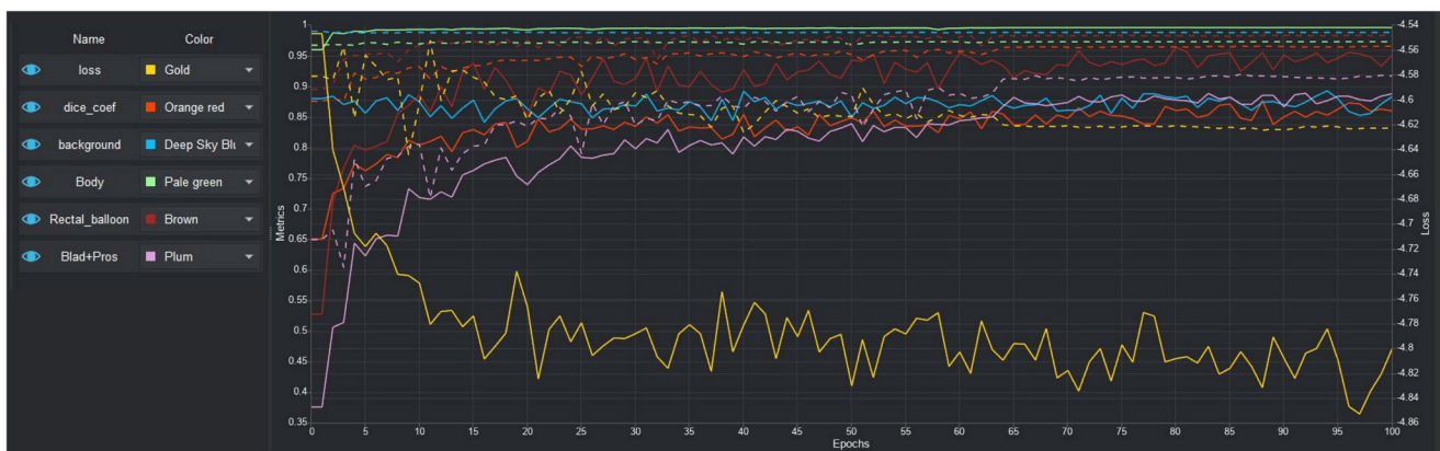
Fig. 4. The training outcome of the fully convolutional DenseNet (FC-DenseNet) model for MVCT auto-segmentation, depicting the fluctuating patterns of dice similarity coefficient for individual regions-of-interest and the overall loss value during 100 epochs of training. MVCT, megavoltage computed tomography.
