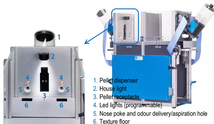
Figure 8. Operon apparatus. On the right, side view of the double-chambered cage (Operon 49500, Ugo Basile S.r.l., Gemonio, Italy), divided by the central sliding door, with an operant stimulation wall mounted on each side. On the left, particular of the stimulation wall (front view) highlighting the position of the following elements: external pellet dispenser (1); house light placed in the top middle of the wall, signalling the length of the punishing timeout (2); central pellet receptacle where precision pellets were delivered (3); programmable arrays of led lights, providing the stimuli belonging to the visual dimension, placed over each nose-poke hole (4); nose-poke holes equipped with the odour delivery/aspiration system, providing the stimuli belonging to the olfactory dimension (5); texture floors, providing the stimuli belonging to the tactile-visual dimension, placed under each nose-poke hole (6).
