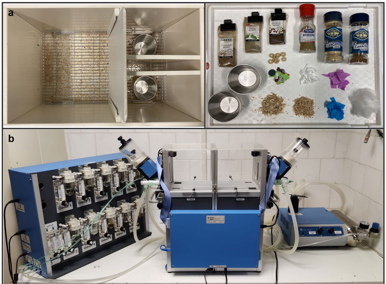
Figure 6. Setting for the manual and automated attentional set-shifting task (ASST) in mice. (a) Photographs of the apparatus for the manual task taken from above (on the left) and of odours and digging media used as stimuli (on the right). (b) Photograph of the apparatus (Operon 49500, Ugo Basile S.r.l., Gemonio, Italy) for the automated task (in the middle), with the odour-delivery unit (on the left) and the pump for the delivery/aspiration system (on the right). In manual ASST, we mixed small amounts of powdered aromatic herbs/spices with the digging media. In automated ASST, odours were prepared by diluting liquid flavours employed in the confectionery industry (5% in mineral oil).
