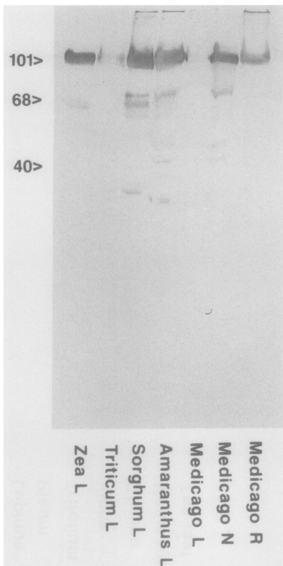
FIG. 7. Nitrocellulose blot of the soluble leaf proteins of various C_3 and C_4 plant species probed with maize leaf anti-PEPC serum. Proteins were electrophoresed in an SDS-PAGE system and then transferred to nitrocellulose. Tissue designations are: L, leaf; N, nodule; R, root. The protein loads are: Zea L, 5 \mu g; Triticum L, 40 \mu g; Sorghum L, 10 \mu g; Amaranthus L, 27 \mu g; Medicago L, 40 \mu g; Medicago N, 36 \mu g; Medicago R, 50 \mu g.
