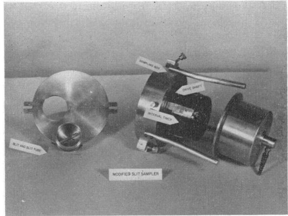
FIG. 4. Component parts of modified slit sampler
