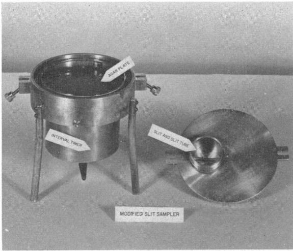
FIG. 2. Modified slit sampler with 150 x 20-mm agar culture plate in position.
