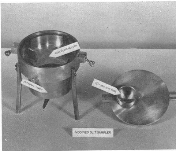
FIG. 3. Modified slit sampler showing assembly of agar plate holder.
