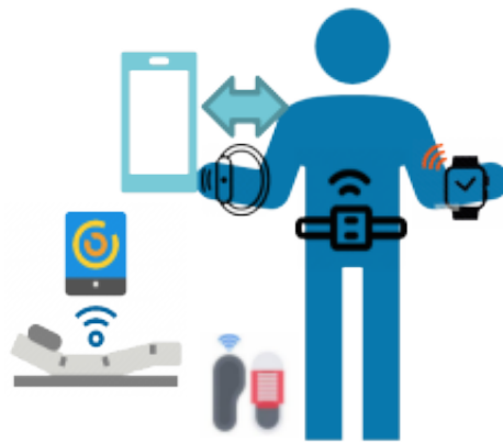
Figure 1. A schematic of the set of wearable devices used in ALAMEDA pilot studies: smart watch, accelerometer bracelet, IMU-sensor belt, ground force sensitive insoles, smart mattress. The figure shows the points on the human body where each device will be worn.
