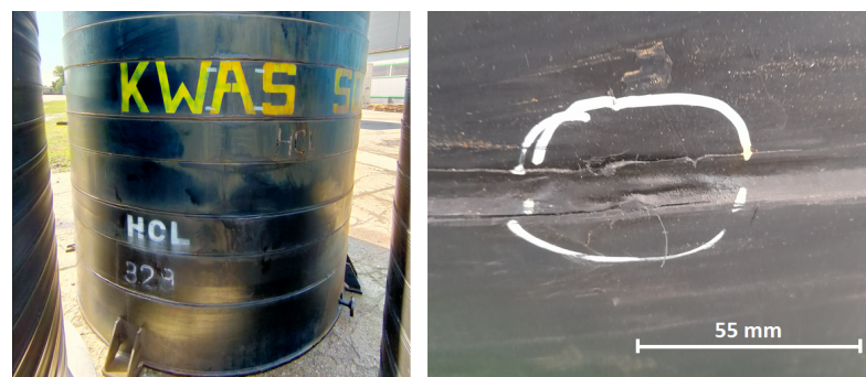
Figure 6. Chemical storage tank for concentrated hydrochloric acid and a crack found in weld of PE layers.
