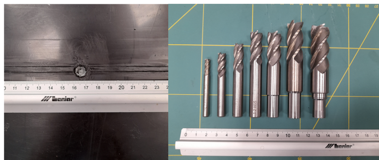
Figure 4. Example of flat bottom hole damage of PE layer and drills used for damage introduction.
