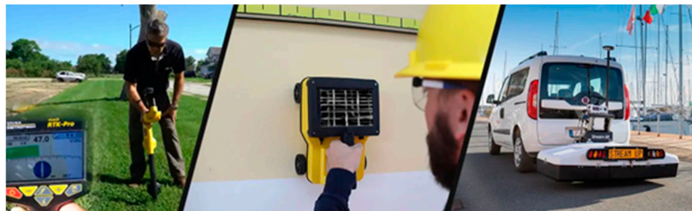
Figure 6. Use of Ground Penetrating radar (Picture courtesy of C R Kennedy Geospatial Solutions).
