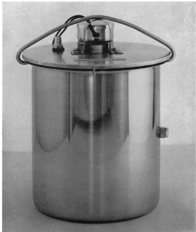
FIG. 1. Agar drum sampler for monitoring airborne bacteria
