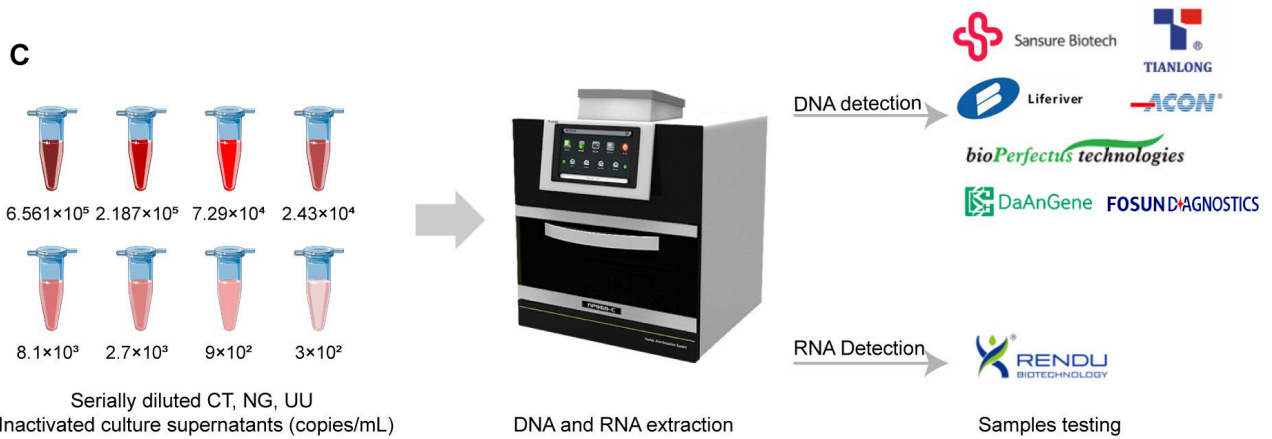
FIG 1 Schematic diagram of the study design. (A) Calculation of amplification efficiency of quantitative PCR. (B) DNA and RNA quantification of CT , NG , and UU inactivated culture supernatants. (C) Evaluation of LODs of DNA-based and RNA-based NAATs.
