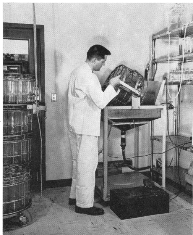
FIG. 2. Stainless-steel funnel with rotatable mount for pouring off fluids. Rubber tubing shown for carrying spent culture fluid to floor drain is replaced with chilled carboy for harvesting infectious fluids.
