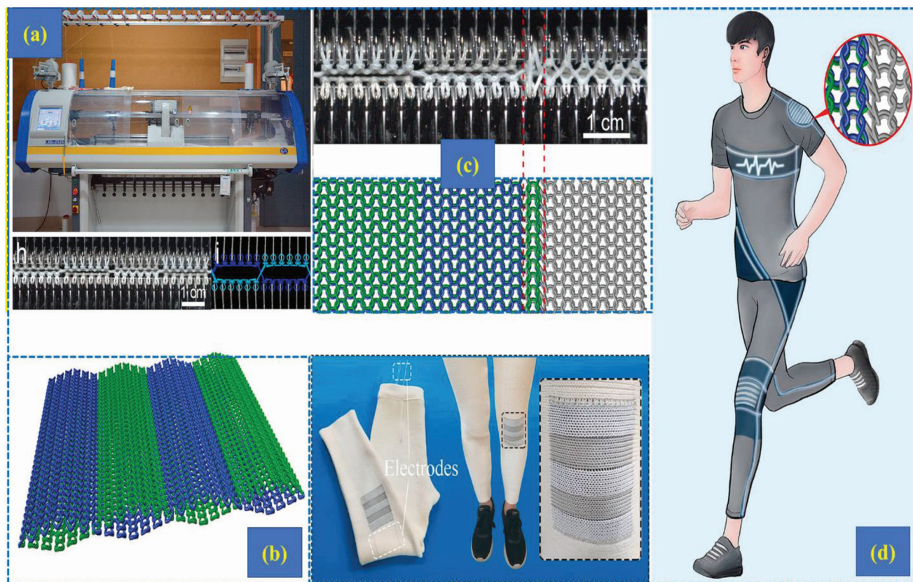
Figure 14. a) Computerized flat knitting machine, b) schematic diagram of knitted T-TEGs samples, c) design and fabrication of the T-TEG samples using a flat knitting machine and d) application of knitted T-TEGs in day-to-day life. Reproduced with permission. [96] Copyright 2020, Elsevier.
