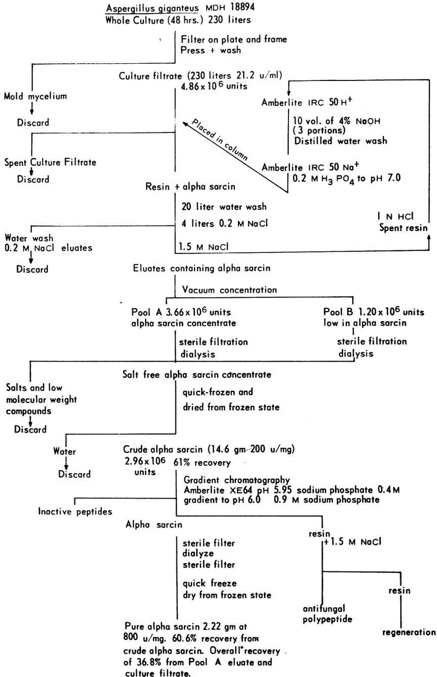
FIG. 1. Isolation and purification procedures for alpha sarcin. Yields from 230 liters of whole culture.
