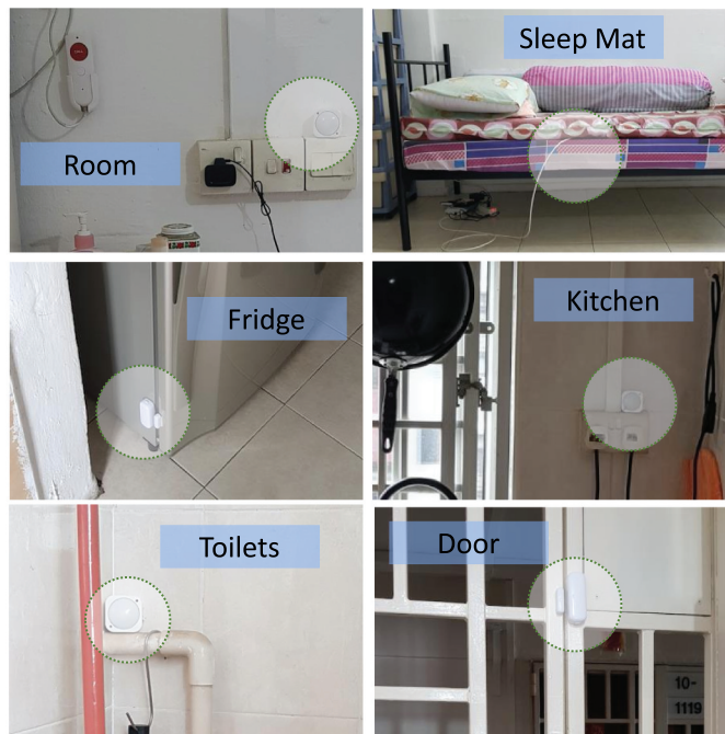
Figure 4. Distribution of the employed sensors in an HDB flat. Motion sensors were located in the living room, kitchen, and bathroom. The contact sensors were located on the main door and the fridge. The bed sensor mat was placed underneath the bed mattress.
