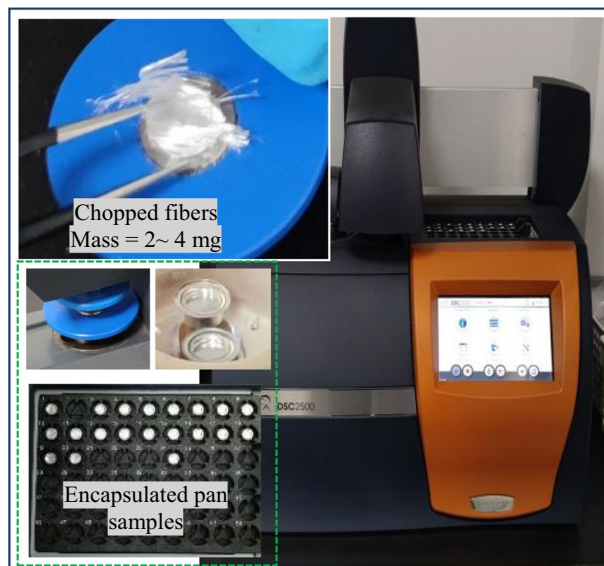
Figure 4. Thermal analysis DSC instrument and chopped fibers.
