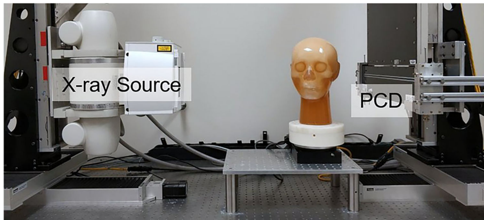
FIGURE 4. Benchtop PCD-CT imaging system used in this work. PCD-CT, photon counting detector CT.
